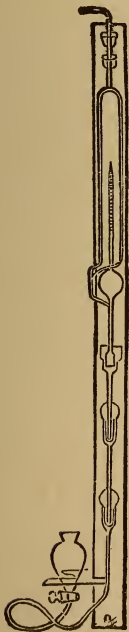
Fig. 101. M'LEOD'S AIR GAUGE, FOR MEASURING PRESSURE DOWN TO ONE TEN MILLIONTH OF ATMOSPHERE.
